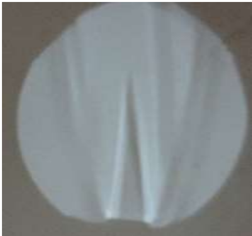
Figure 4. The flame form using the Schlieren method.
